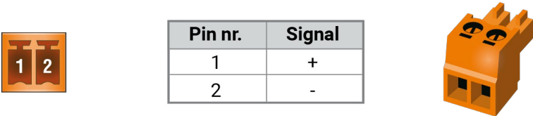
2-pole Phoenix connector and plug pin assignments
